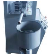
Fig. 5 Pot winder with adjustable drive motor
