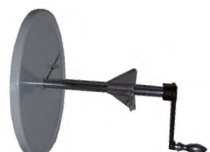
Fig. 8: Spool winding axle with hand crank
