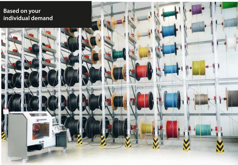
Fig.1 LAGROL drum rack with MOTROL 800 EASY coil and spool winding machine
