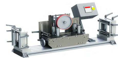
Fig. 1 MESSBOI 80 LC with housing and roller cages on alu profile
