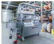
Fig. 4 AUTOCUT 40 with open protective cover
