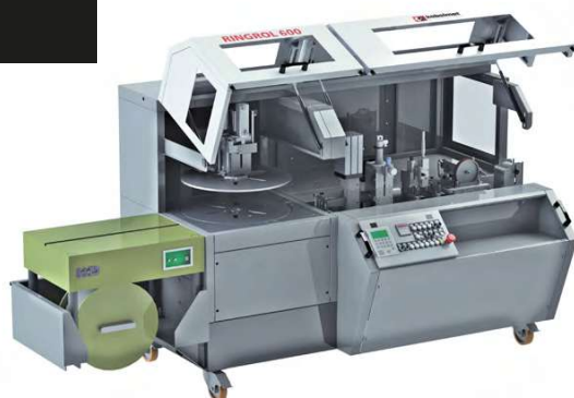
Fig. 1 RINGROL 600 with open cover and binding device
