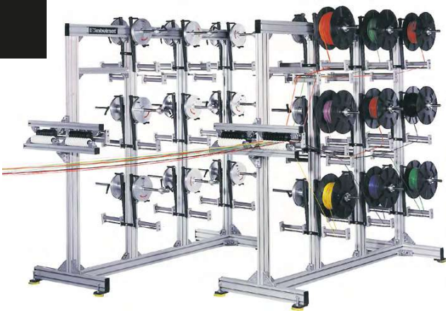
Fig. 1 SPULROLLY example for arrangement with split pair coils
