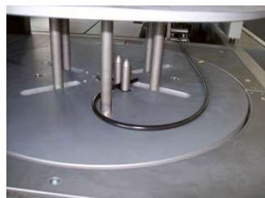
Fig. 4 Cable fixing clamp for winding plate
