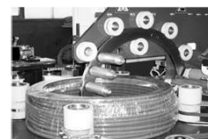
Fig. 8 Wrapping station for stretch straps
