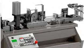
Fig 4 Central adjustment of the guide rollers optional motor driven version available
