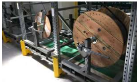
Fig. 3 TROMTRAK 1000 drum storage device in use
