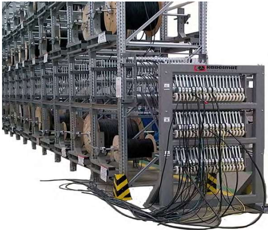
Fig. 2 TROMBULLY with central point of removal and return stop
