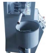
Fig. 5 Pot winder with adjustable drive motor
